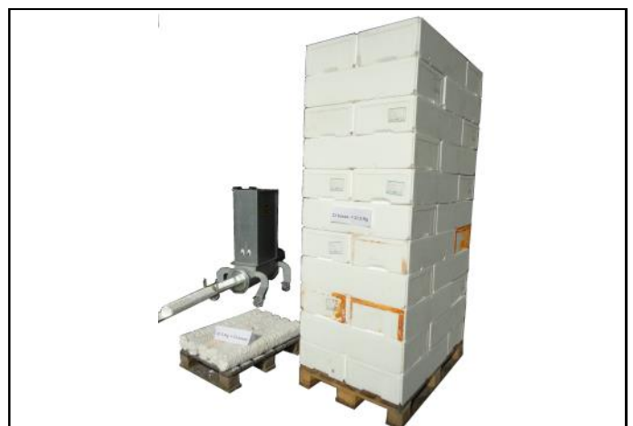
The Styropactor NANO or "Styrofoam Bug" illustrating 33 non-compacted and 33 compacted fishboxes.
